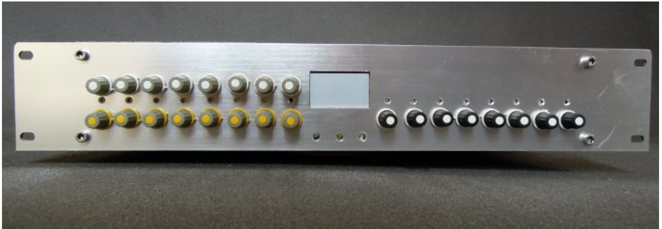
All the circuitry is mounted in a standard 19inch chassis. The unit can be screwed into a rack for easy transport.
